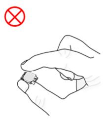
When handling the product, do not apply direct pressure on the resin.
